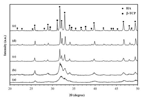
Figure 2. Patterns of XRD analysis related to natural HA of thermal analysis at temperatures of: (a) 400°C (bone ash); (b) 600°C; (c) 700°C; (d) 900°C and (e) 1100°C.
