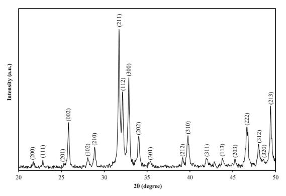
Figure 6. All of the diffraction planes of HA firing at 900°C.
