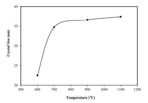
Figure 4. Crystal size (nm) of HA against firing temperature.
