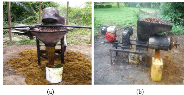
Figure 2. Various early designs of palm oil press in use in Cameroon; manual (a) and motorized (b).
