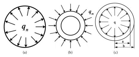
**Figure 1.** Stress model of anchor solid and surrounding rock. (a) Internal force of borehole surrounding rock; (b) Anchor body subjected to external force; (c) Internal force on anchor body.
