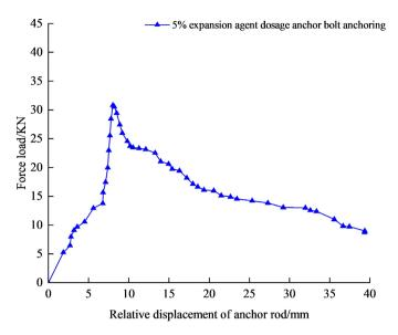
**Figure 5.** Changes in axial load displacement curve of anchorage with 5% expansion agent content.
