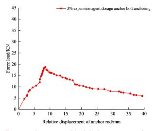
Figure 4. Changes in axial load displacement curve of anchorage with 3% expansion agent content.
