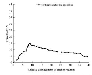
Figure 3. Changes in axial load displacement curve of ordinary cement anchorage.
