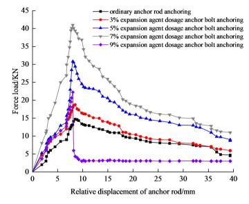
**Figure 9.** Comparison of axial load curves for anchor bolts with different pressurization sizes.
