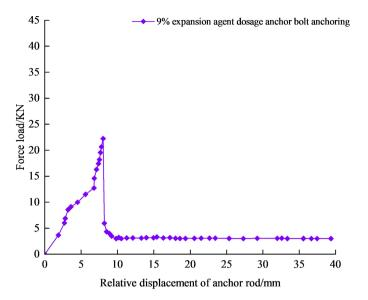
**Figure 7.** Axial load displacement curve variation of 9% expansion agent dosage anchoring.
