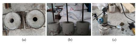
**Figure 2.** Experimental steps. (a) Preparation of test blocks; (b) Anchor rod anchoring; (c) Anchor rod pulling.
