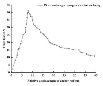
**Figure 6.** Changes in axial load displacement curve of 7% expansion agent content anchorage.
