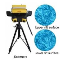
**Figure 4.** OKIO-400 laser scanner (left), 3D model of nodal surface (right).
