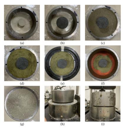
Figure 5. Specimen encapsulation process.
