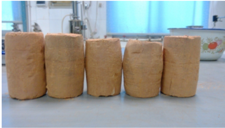
Figure 6. Soil samples of saturated red clay after consolidated drained test.
