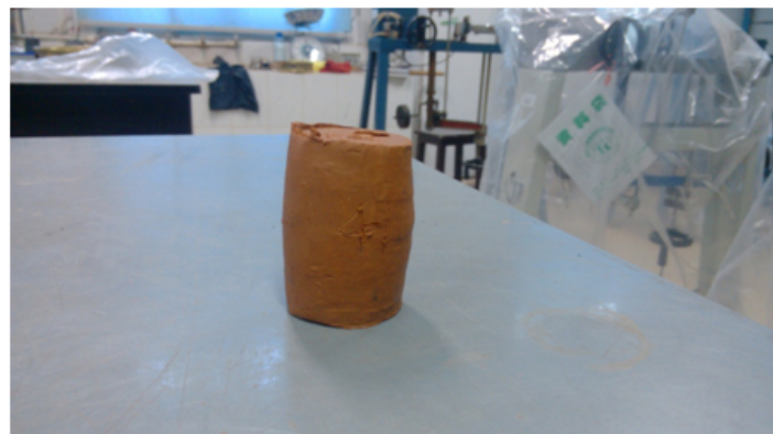
Figure 17. Bulging deformation of soil samples with moisture higher than 35%.
