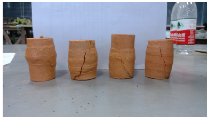
Figure 16. Shear failure of soil samples with moisture content below 35%.
