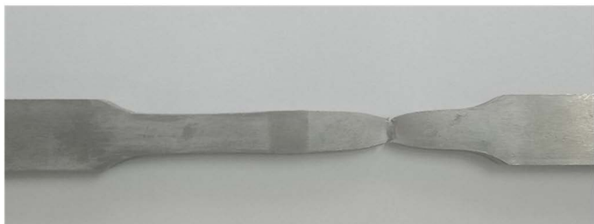
Figure 12. Macrographs showing fractured location in the tensile specimen.
