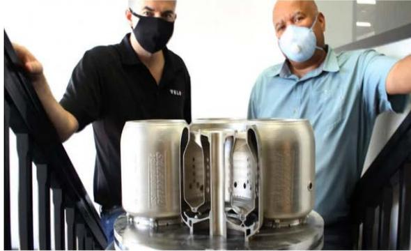
**Figure 4.** Sierra turbines via AM.
