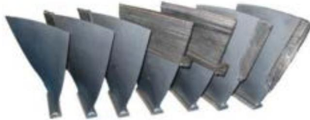
**Figure 6.** The repaired turbines via AM.
