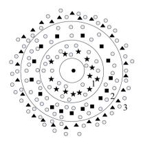
Figure 1. System model of ring routing strategy between clusters.
