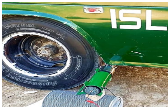
Figure 5. Device attached to exhaust of a diesel bus.
