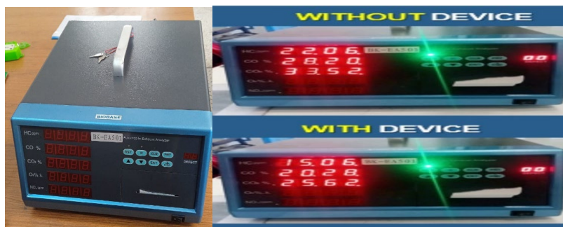
Figure 10. Gas analyzer BK-EA501 showing HC, CO and CO 2 emissions.
