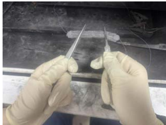
Figure 3. Schematic illustration of the practical stretching operation using laboratory tweezers.
