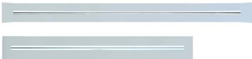
Figure 2. The lower section indicates the sensor's length in the relaxed state; the upper section demonstrates its length change under stretching.
