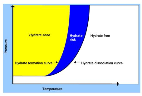
Figure 1. Typical hydrate formation diagram.
