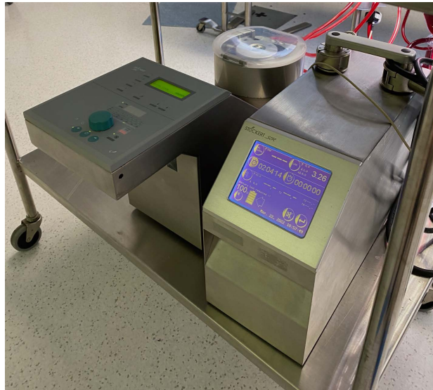
Figure 1. Modified cardiopulmonary bypass circuit consisting of a Sorin/Stöckert SCP centrifugal pump (LivaNova PLC, London, United Kingdom) and Medtronic (Medtronic Inc., Minneapolis, MN) tubing and reservoir.
