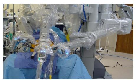
Figure 4. Side docking of the robot.
