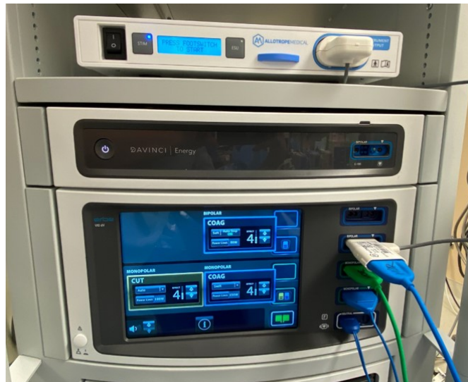
Figure 1. StimSite signal box connected to surgical instrumentation. STIM button is pressed when ready to visualize the ureter, and dedicated foot pedal used to deliver the fixed signal.
