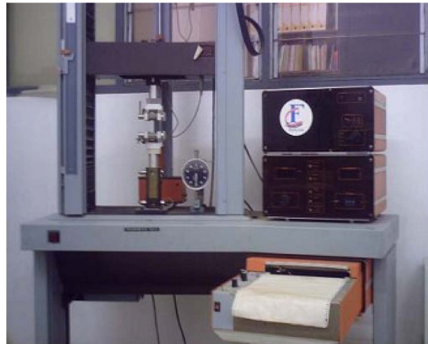
Figure 10. Lab dynamometer for tensile testing of rubbers.
