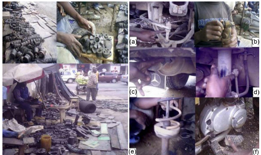
Figure 2. Auto parts made from used tires include silent-blocks ((a), (b), (d)), an exhaust support clamp (c), a wedge for reinforcing the tie rod (e), and the brake pedal and footrest of a motorcycle (f). (Photo credit: authors)
