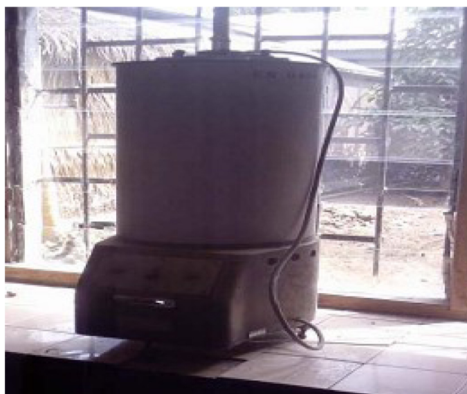
Figure 12. Lab air-oven for thermo-oxidative ageing of rubbers.
