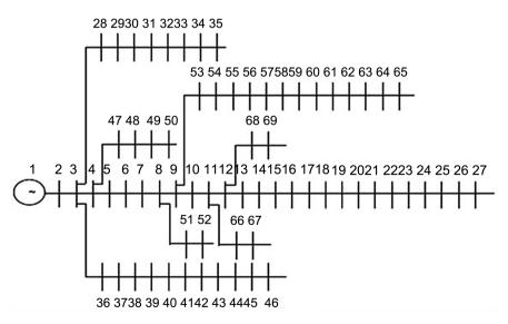
Figure 3. Single-line diagram of 69-bus system.
