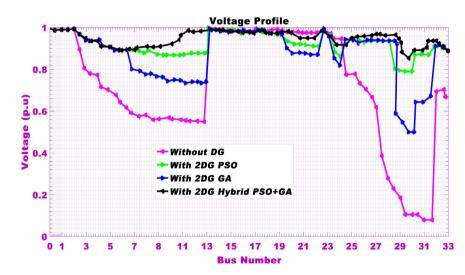
Figure 6. Voltage profile at IEEE 33-bus.
