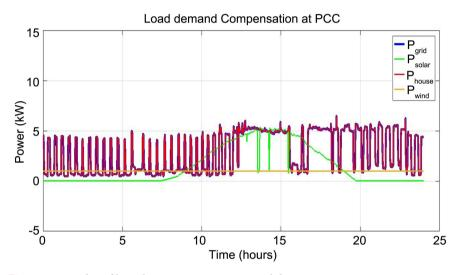
Figure 10. Load profile and power compensation with battery.
