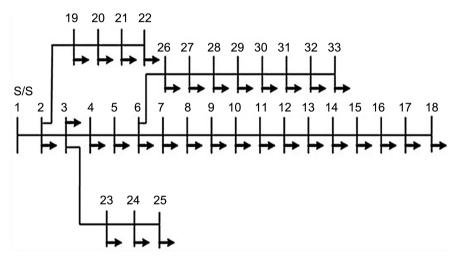
Figure 2. Single-line diagram of 33-bus system.
