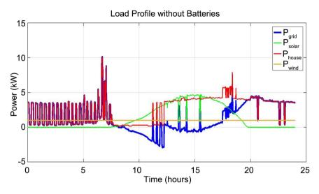
Figure 8. Load profile and power without battery.
