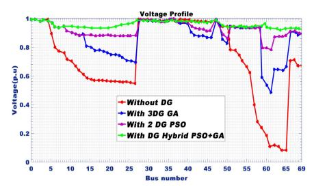
**Figure 7.** Voltage profile at IEEE 69-bus.
