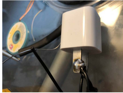
Figure 7. iPhone USB charger connected to white and black neutral wires. The charger is used as a power source for the raspberry pi zero w.
