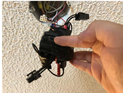
Figure 8. Device and all of its components are in compaction. The electrical tape is used as a case to consolidate all the components which makes the device take up less space minimizing the amount of space the device takes up.
