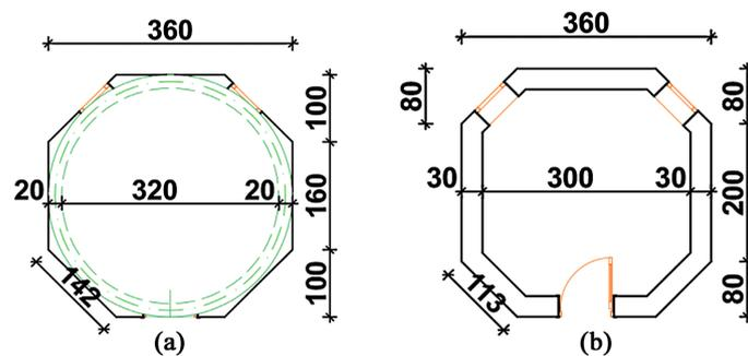
**Figure 2.** (a) Plan view of house with dome; (b) Plan view of house without dome.
