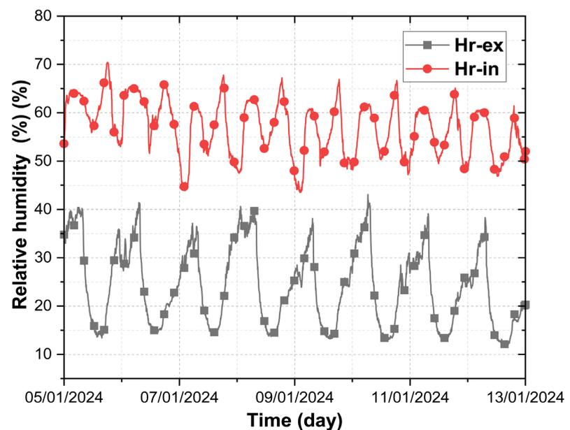
**Figure 9.** Relative humidity of internal and external environments from 05/01/2024 to 08/01/2024.
