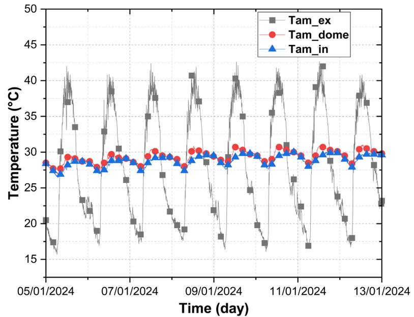
**Figure 6.** Internal and external ambient temperature profile for the period 05/01/2024 to 08/01/2024.
