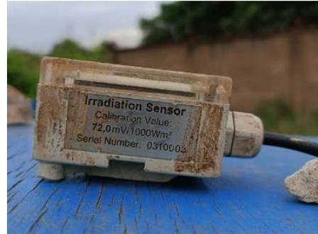
**Figure 3.** Solarimeter.
