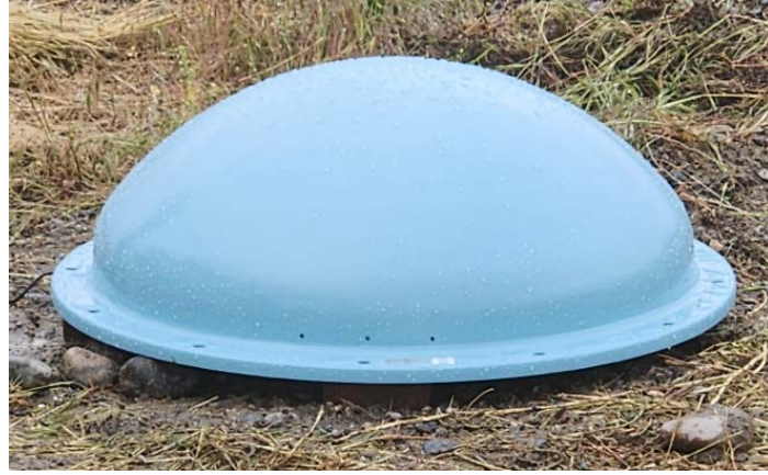
Figure 1. The fiberglass hemispherical radome is leveled and centered over the GPS antenna.
