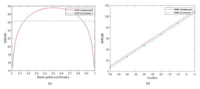
Figure 3. (a) Effect of beam splitting ratio on SNR; (b) Effect of signal optical power on SNR.
