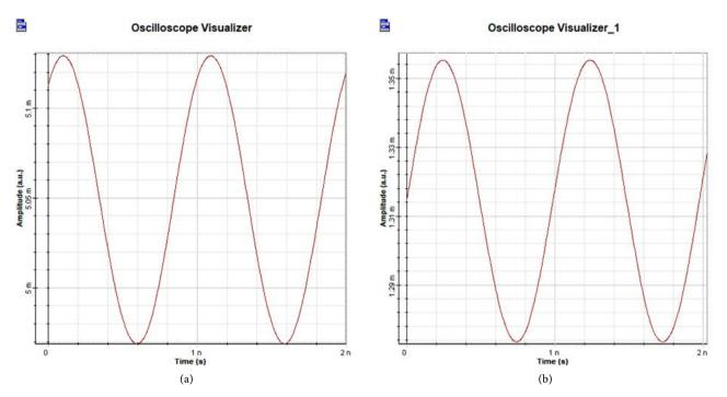
**Figure 8.** The 1/4 glass plate changes from a 45° polarization angle to a 20° polarization angle, the phase difference of signals in channel (a) and (b) is not equal to  $\pi/2$  and the SNR was reduced by 2 dB.
