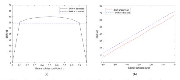
Figure 5. (a) The influence of beam splitting ratio on SNR; (b) Simulation diagram of the influence of signal optical power on SNR.
