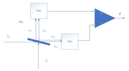
Figure 1. Schematic diagram of balance detection.
