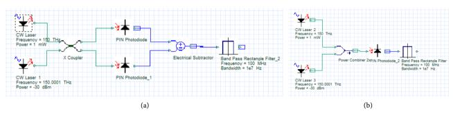
Figure 4. (a) Balance detection simulation diagram; (b) General heterodyne detection simulation diagram.
