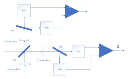
Figure 2. Schematic diagram of double balance detection.
