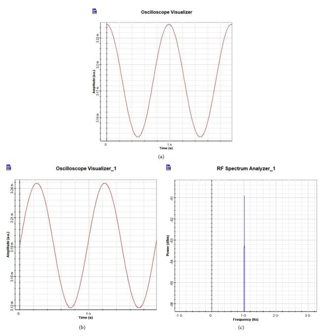
**Figure 7.** (a) is in-phase component (I) and (b) is quadrature component (Q), the simulation results that the phase difference of the components of system I and Q is  $\pi/2$ . (c) Difference frequency signal frequency domain waveform.
