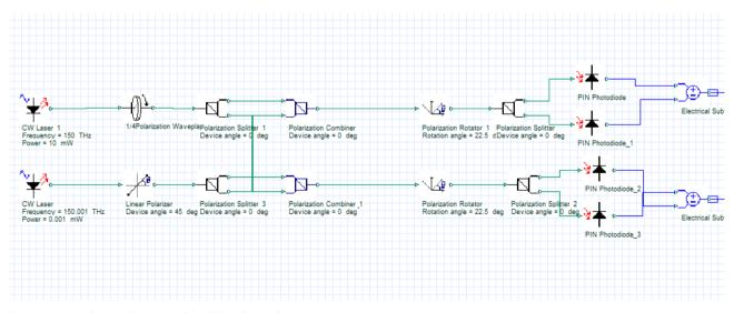
Figure 6. Simulation diagram of double balance detection.
