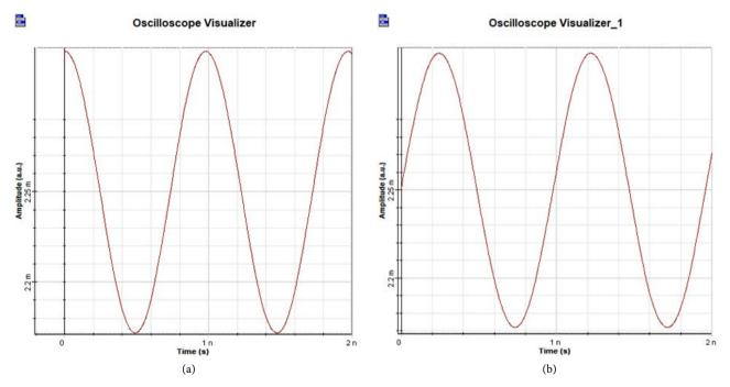
Figure 9. The 1/2 glass slide was changed from 22.5° to 30°, the SNR was reduced by 3 dB (from 41 dB To 38 dB).
