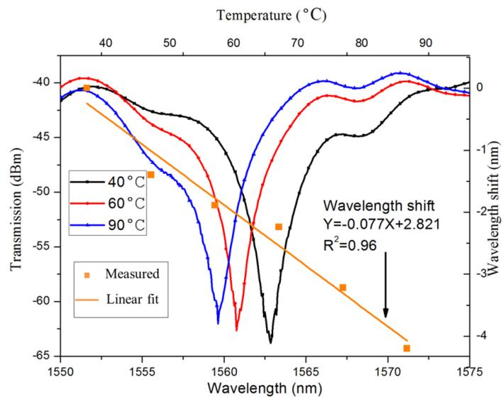
**Figure 5.** Measurement results of SMS temperature.
