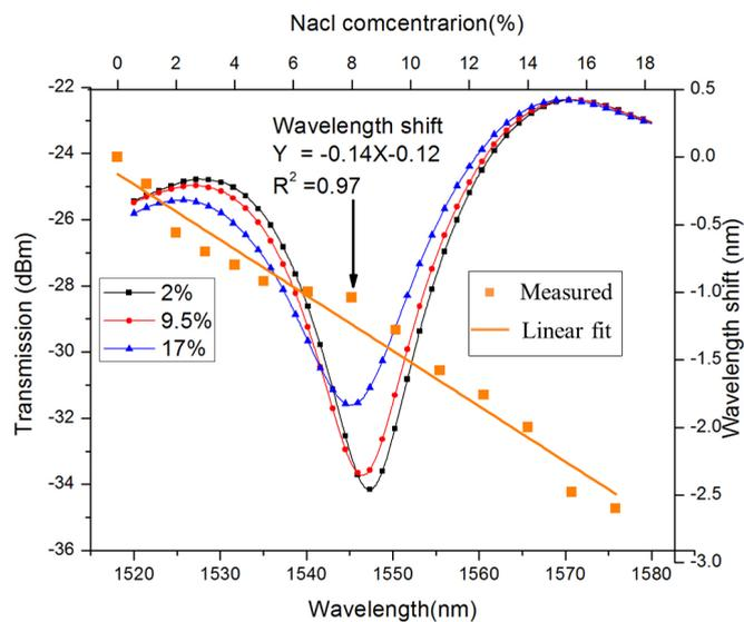
**Figure 2.** Measurement results of LPFG concentration.
