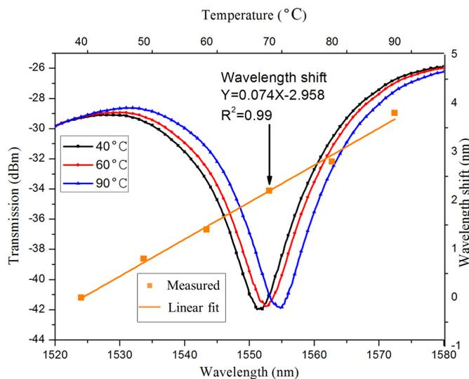
**Figure 3.** Measurement results of LPFG temperature.
