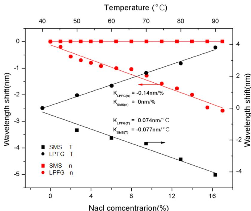
**Figure 6.** Cascade of sensitivity parameters for LPFG and SMS.
