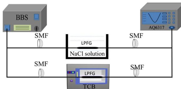
**Figure 1.** Measurement structure of LPFG temperature and concentration.
