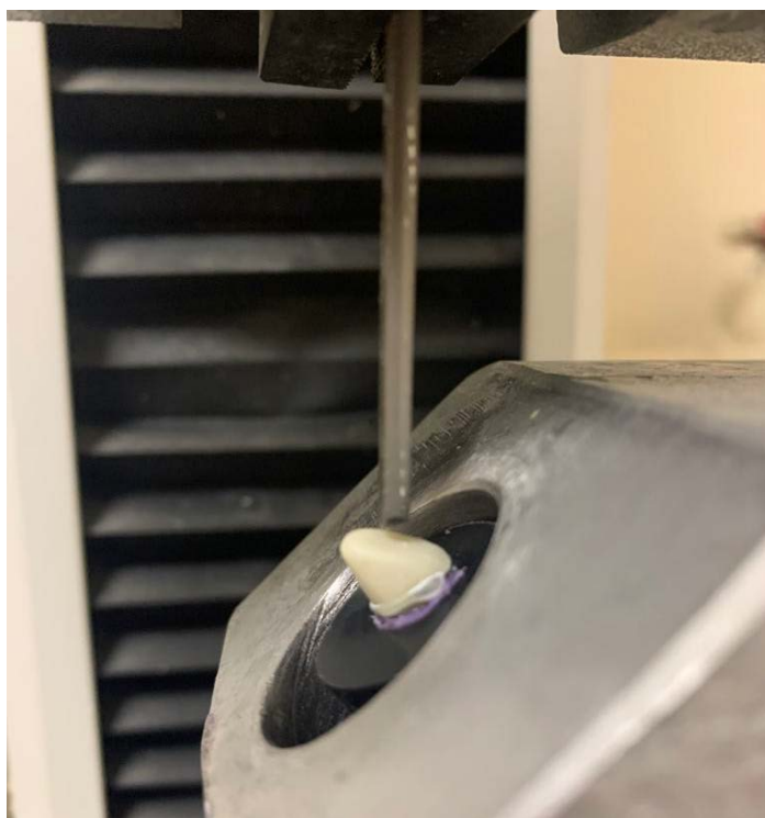
Figure 1. Fracture strength test.
