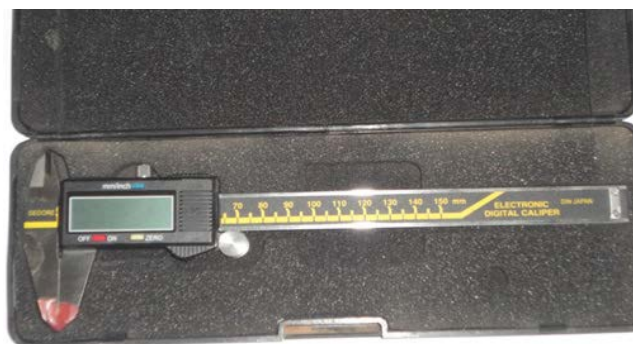
Figure 1. The digital caliper is calibrated in millimeters and inches. It is 150 mm in length. The peripheral end is fixed, while the other one is sliding used to adjust the measurement. Made in China.
