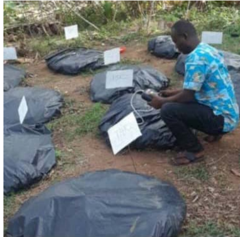
Figure 2. GHGs emissions measurements using the Infrared Gas Analyzer.
