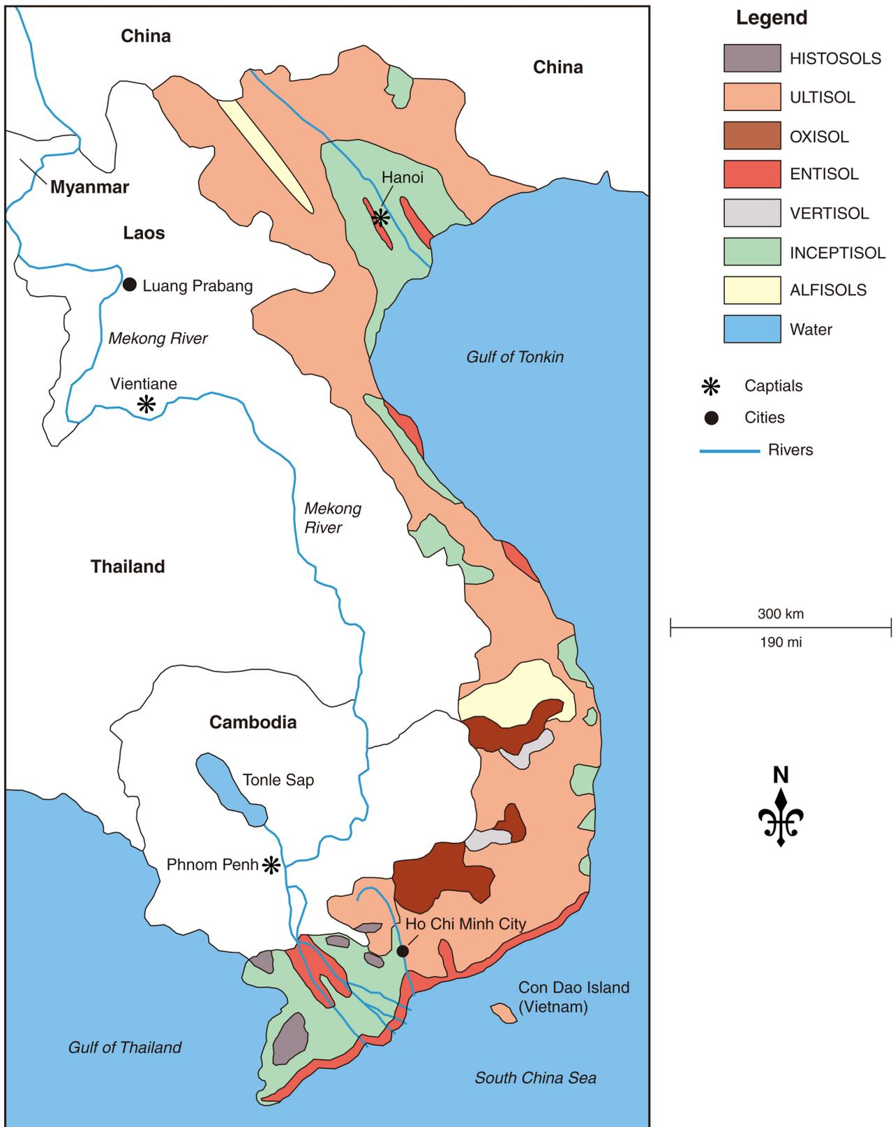
**Figure 25.** Soil map of Vietnam. Based on FAO/UNESCO [preliminary definitions, legend and correlation table for the soil map of the world. World Soil Resources Report no. 12. Map by Mic Greenberg. Reprinted with permission from Open Journal of Soil Science 2019, 9: 1-34. Published with copyright permission from Editor of Open Journal of Soil Science.
