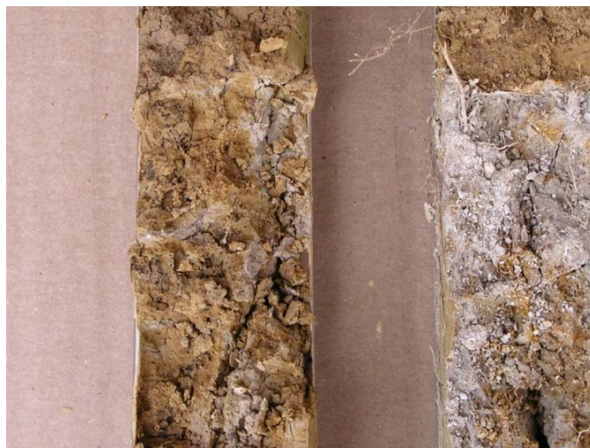
Figure 1. Fragipan cores untreated (left) and treated with sodium fluoride (NaF) and annual ryegrass (ARG) after one year.
