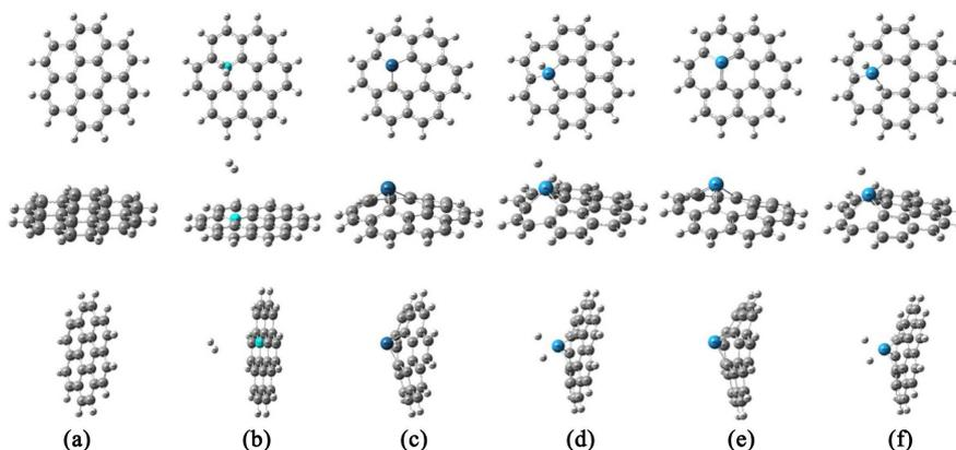
**Figure 2.** The optimized structures of (a) pure GS; (b)  $\text{H}_2$ @GS; (c) Os-GS; (d)  $\text{H}_2$ @Os-GS; (e) W-GS and (f)  $\text{H}_2$ @W-GS.
