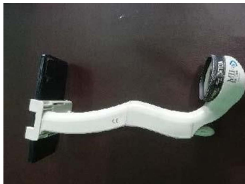
Photo 1. MII Ret Cam device coupled to the smartphone and the volk 20 diopter lens.
