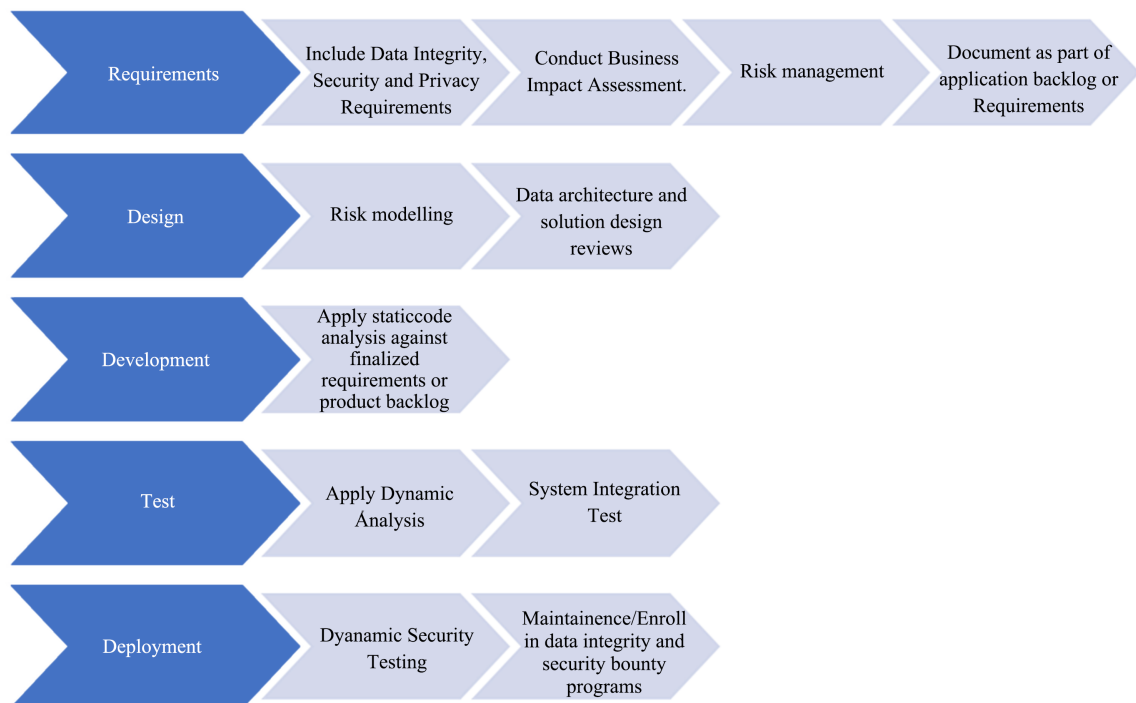
Figure 1. Basic DIaC framework that can be used as a starting ground for product development teams.
