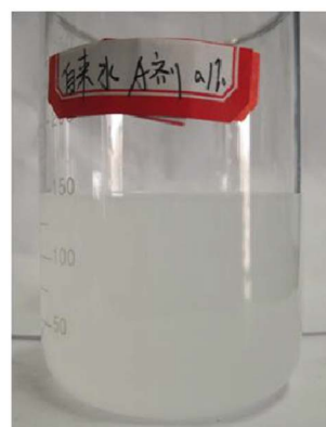
Figure 2. Slippery water fracturing fluid prepared by agent A and agent B.
