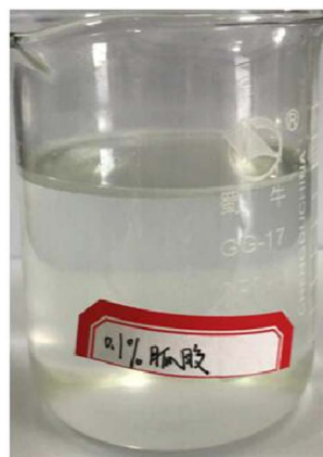
Figure 3. Slippery water fracturing fluid formulated with guar gum, drainage aid and demulsifier.
