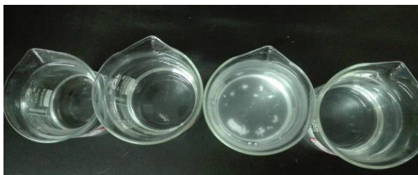
Figure 2. Dissolution of blank, CQFR drag reducer, oil-based emulsion drag reducer, powder drag reducer in ①.
