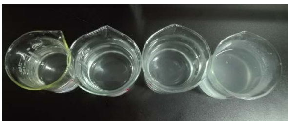
Figure 3. Dissolution of blank, CQFR drag reducer, powder drag reducer, oil-based emulsion drag reducer in ②.
