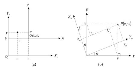
**Figure 3.** Schematic diagram of translation and rotation of coordinate systems. (a) Translation; (b) Rotation.
