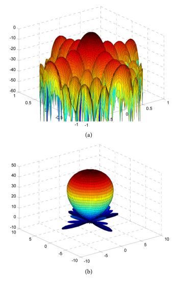
**Figure 9.** Transponder's antenna pattern. (a) Directional cosine coordinate system; (b) Spherical coordinate system.
