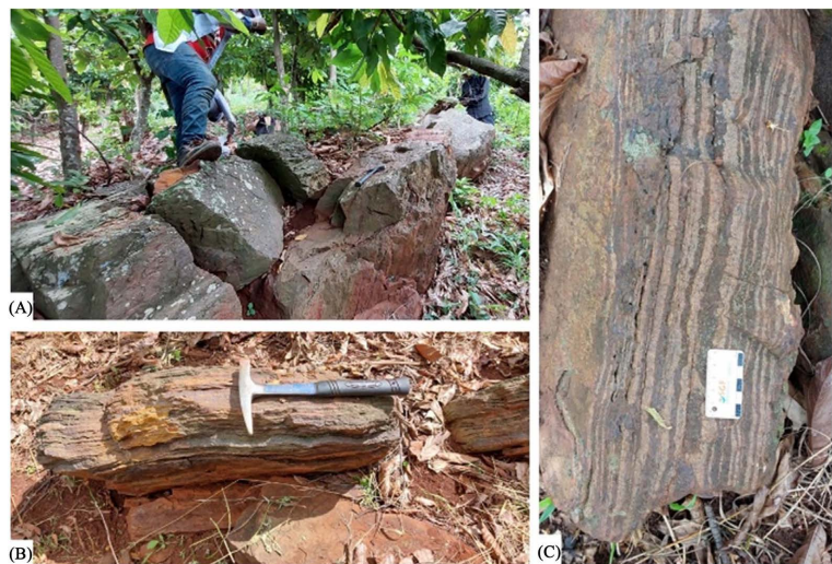
Figure 10. Magnetite-rich quartzites: (A) outcrop of BIF; (B) BIF oxidized to hematites, goethite and limonite; (C) Alternation of magnetite beds (hematites) and silica beds.
