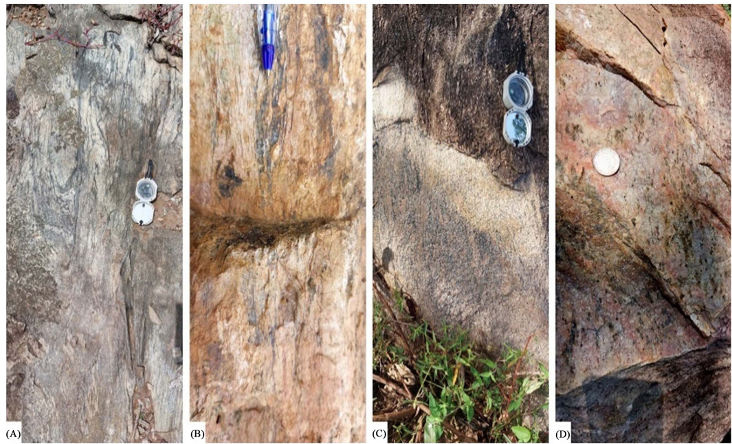
Figure 21. Mylonitic formation of shear zones: (A) Orthogneiss proto mylonite, (B) Orthogneiss mylonite, (C) Pegmatitic granite protomylonite, (D) Pegmatitic granite mylonite.
