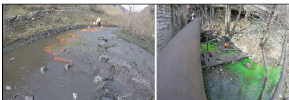
Figure 6. To the left: Indicative experiment of water marking carried out in the polluted bed of the Rganisghele River. To the right: Dyed stream observed in the drinking water of the Monastery spring.
