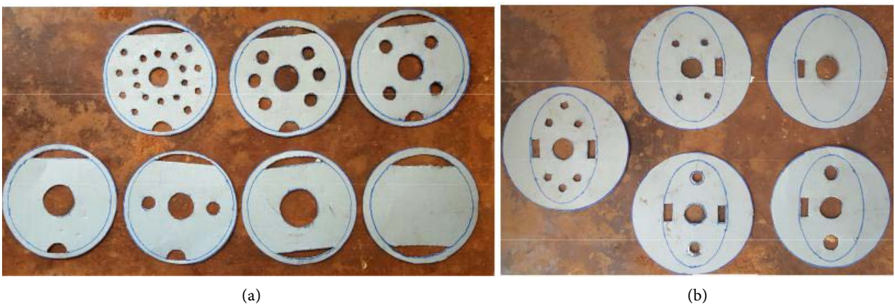
Figure 25. (a) Cylindrical tank Baffle test pieces, (b) Elliptical tank Baffle test pieces.
