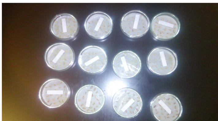
**Plate 1.** Germination seeds test arrangement in groups of 25, on moistened filter paper.
