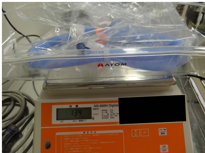
Figure 2. A digital infant scale (NS-608N Digital Infant Scale, Atom Medical Corp. Tokyo, Japan) was used to weight condensation. The difference before and after ventilating the circuit was determined as the amount of condensation generated.
