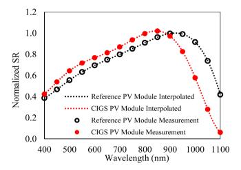
Figure 17. Spectral responsivity of CIGS\_1 PV module.
