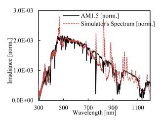
**Figure 3.** Spectral distribution of simulator versus AM1.5 at 200 Wm<sup>-2</sup>.
