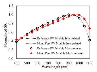
Figure 16. Spectral responsivity of MonoPerc PV module.
