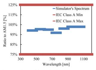
**Figure 4.** Evaluation of the simulator's spectrum versus AM1.5 at  $1000 \text{ Wm}^{-2}$ .
