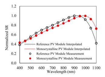
Figure 14. Spectral responsivity of monocrystalline PV module.
