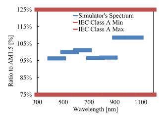
**Figure 5.** Evaluation of the simulator's spectrum versus AM1.5 at 200 Wm<sup>-2</sup>.
