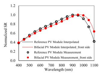
Figure 15. Spectral responsivity of bifacial PV module.
