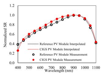
Figure 18. Spectral responsivity of CIGS\_2 PV module.
