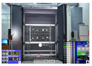
Figure 1. Thermal chamber integrated solar simulator system.
