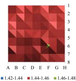
**Figure 6.** Non uniformity measurement of solar simulator as a function of irradiance at 1000 Wm<sup>-2</sup>.
