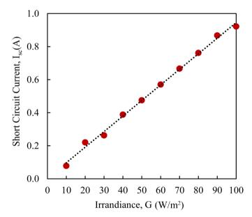
**Figure 12.** *I*<sub>sc</sub> - *G* curves of a monocrystalline PV module.
