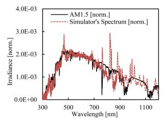
**Figure 2.** Spectral distribution of simulator versus AM1.5 at 1000 Wm<sup>-2</sup>.
