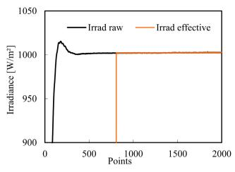
Figure 9. Temporal instabilities of solar simulator regulated by control cell.
