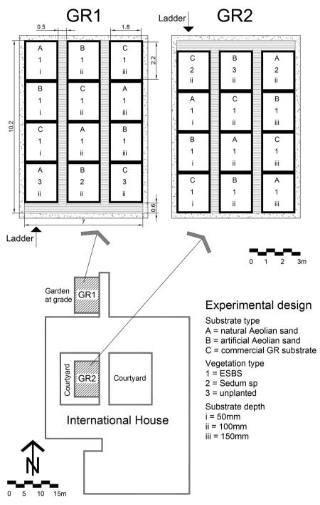
**Figure 6.** Experimental design for the ESBS green roof project at International House, University of New South Wales [104].
