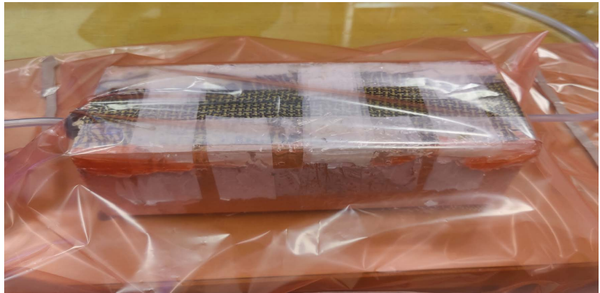
Figure 6. Experimental setup for VARTM process.
