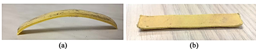
Figure 6. (a) Test sample printed without P-surface 141; (b) Test sample printed on P-surface 141
