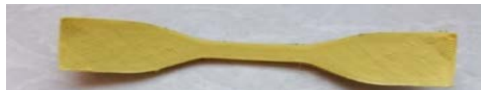
Figure 7. Tensile test sample printed from the rHDPE/TPS composite filament.
