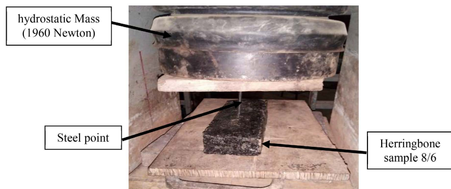
Figure 5. Monnin hardness measuring device.
