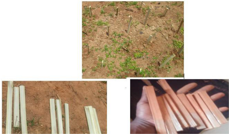
Figure 9. BV3 before and after natural durability test.
