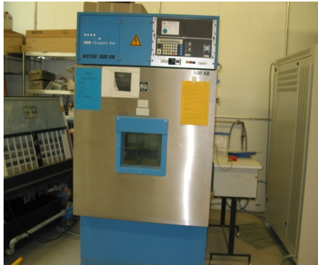
Figure 1. Climate chamber for the sorption experiment. Model: Weiss 500 SB ; Temperature range: +10°C to +95°C; Humidity range: 15% to 98% R.H; Chamber dimension: 850 × 795 × 800 mm (B × D × H).
