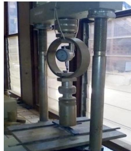
**Figure 8.** 3-point bending test machine.
