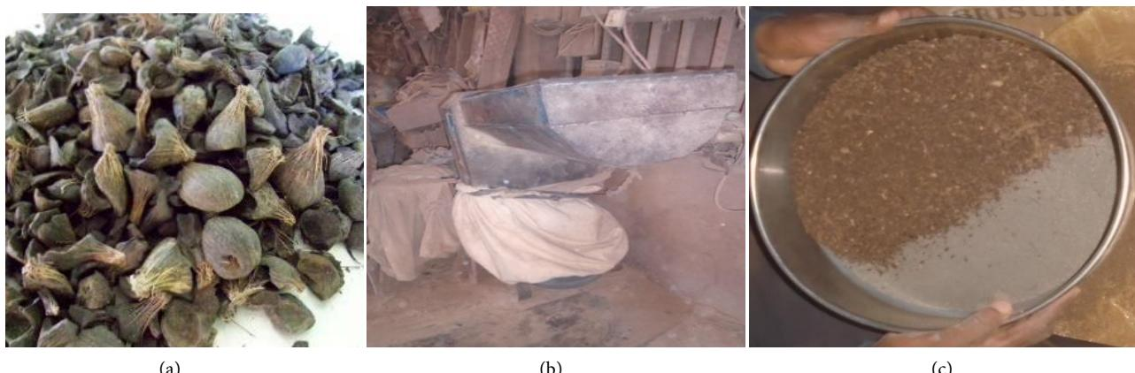
**Figure 5.** Some steps to get palm nut particles. (a) Palmist shell (b) Mulcher of palm kernels (c) Sieving of crushed palm shells.
