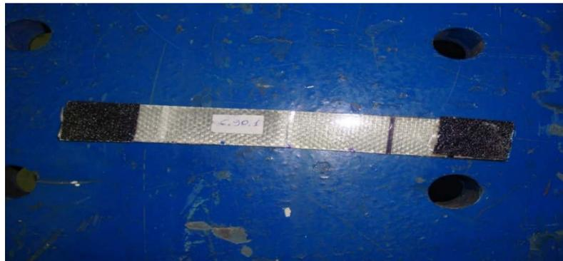
**Figure 10.** Characteristic failure type of coupons with 90° fiber orientation.
