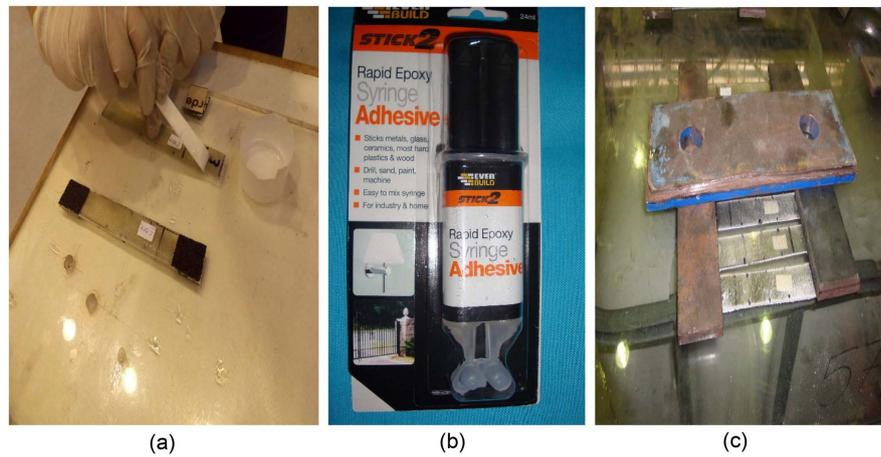
**Figure 6.** Placement of tabs. (a) Applying epoxy; (b) Epoxy glue used for the placement of the tabs; (c) Applying weight to ensure uniform spreading of epoxy.
