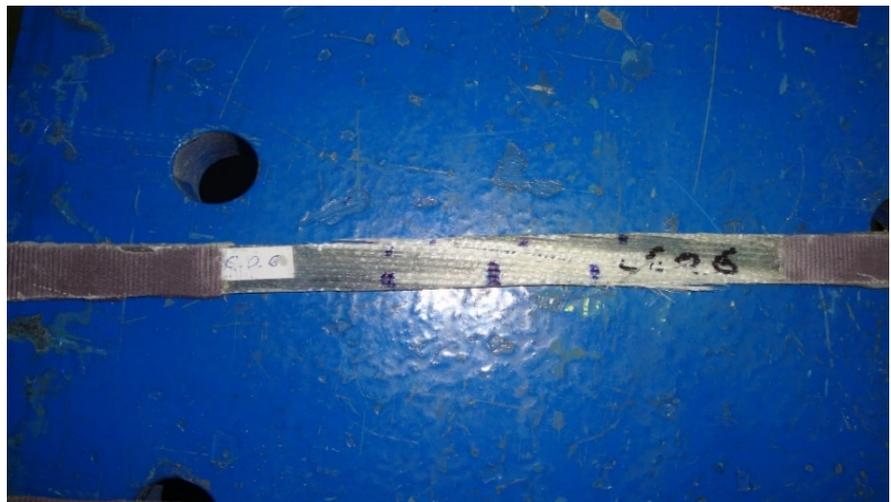
**Figure 8.** Characteristic failure type of coupons with 0° fiber orientation.
