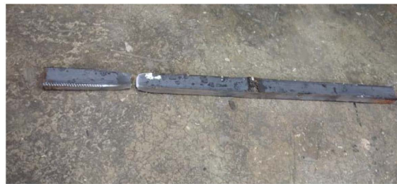
Figure 2. Samples of weld joints after testing.
