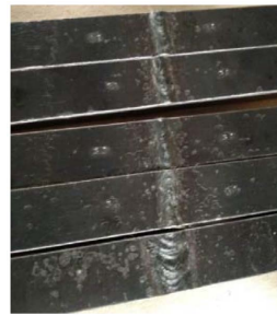
Figure 1. Construction steel specimens prepared for impact toughness testing.
