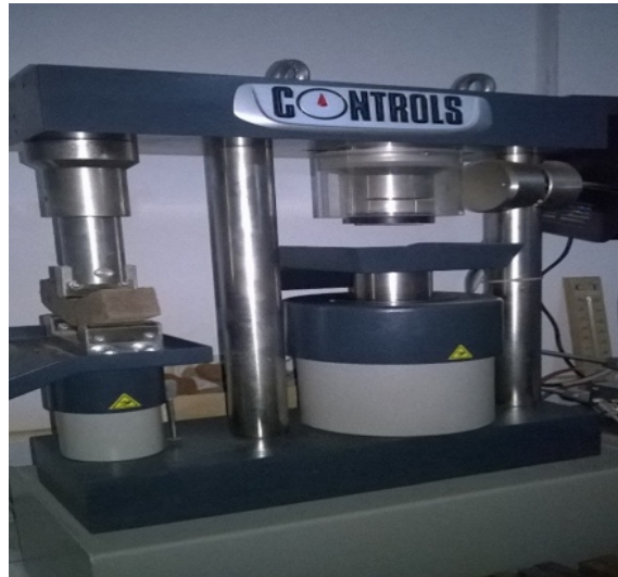
Figure 16. Simple compression and bending tests.
