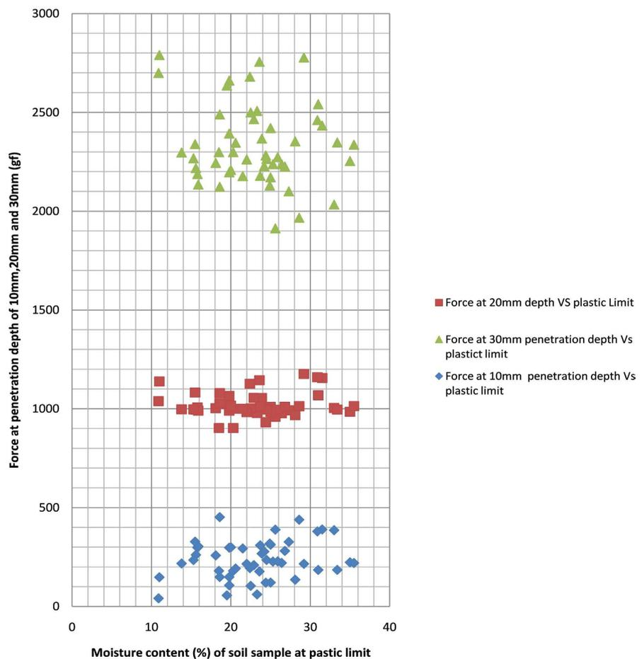
**Figure 7.** Showing a graph of force at penetration depth of 30 mm, 20 mm and 10 mm against moisture content of soil samples at plastic limit.
