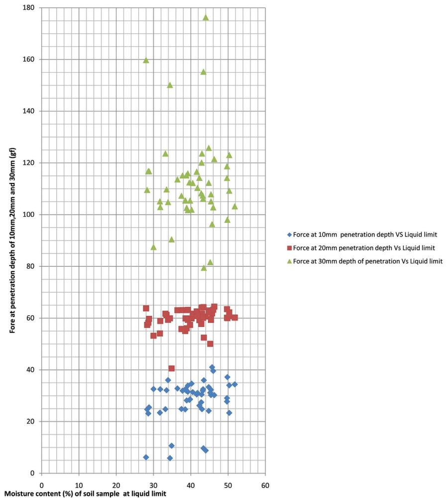
**Figure 8.** Showing a graph of force at penetration depth of 30 mm, 20 mm and 10 mm against moisture content of soil samples at liquid limit.
