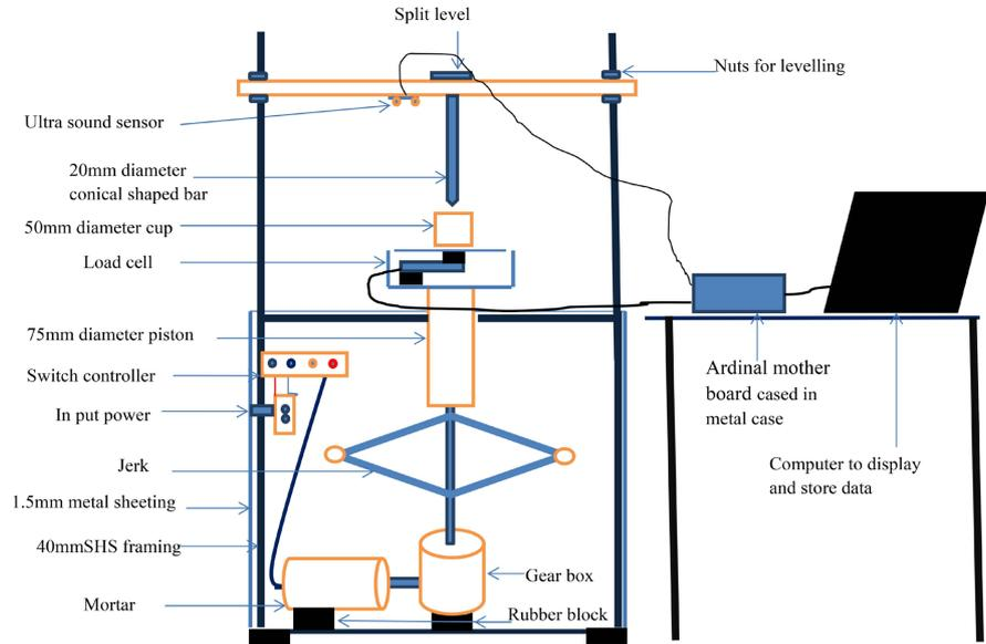
Figure 2. Shows systematic drawing for quasi static machine.
