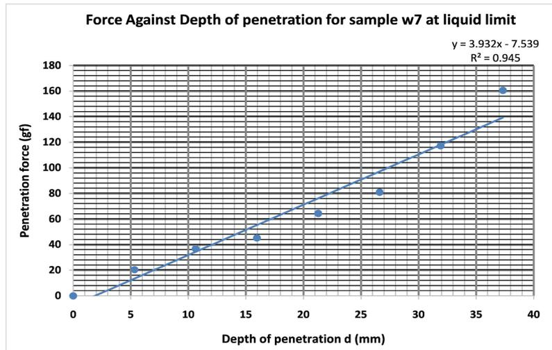
Figure 4. Shows a graph of force against depth of penetration at Liquid limit.
