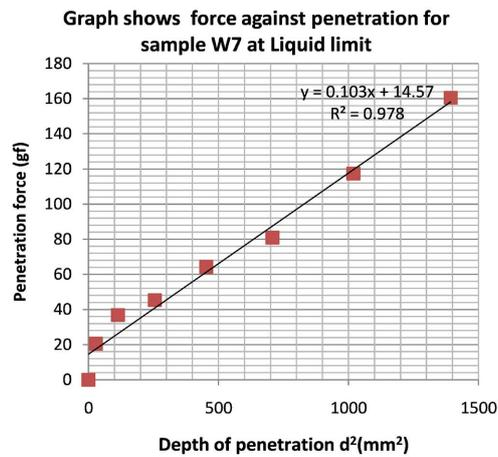
Figure 6. Force against depth of penetration squared at Liquid limit.
