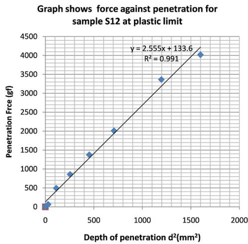
Figure 5. Force against depth of penetration square at plastic limit.
