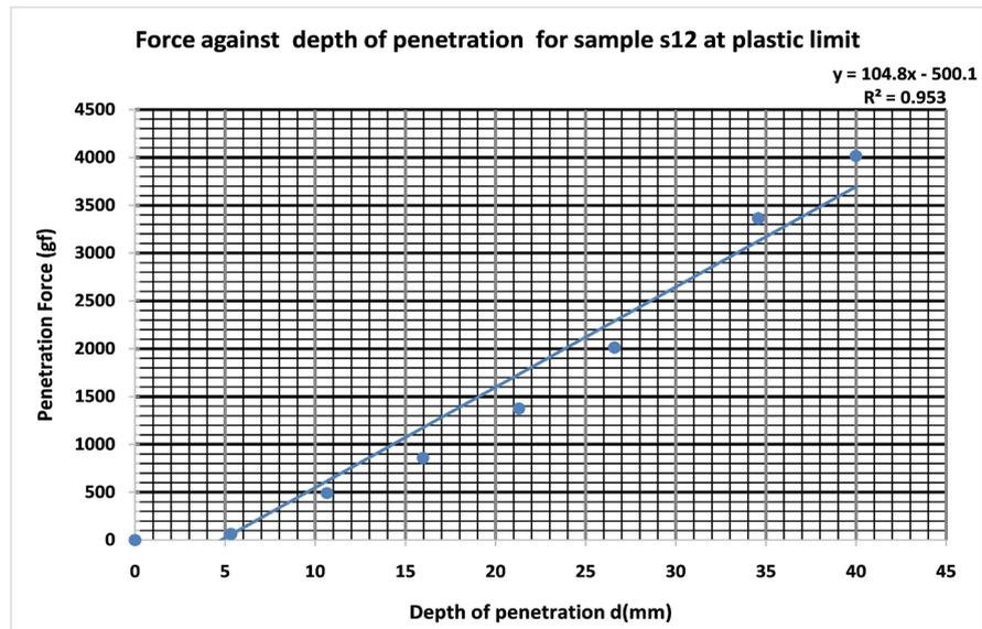
Figure 3. Shows a graph of Force against depth of penetration at plastic limit.
