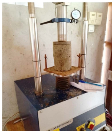
Figure 3. Compression test on GRH-A.
